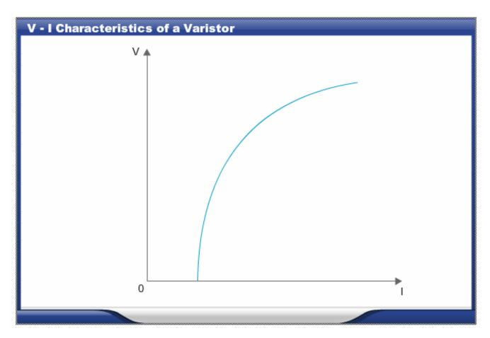
Varistors made of metal oxides are mostly used to provide protection against high voltage surges caused in the transmission and distribution systems by lightning where the voltage surge appears in micro seconds. The lightning current could be discharged in micro seconds if resistance in the discharge path is reduced in time. Varistors are capable of giving this reduced resistance value when voltage increases. By discharging the surges thus, the interruption in the electricity system is averted.
