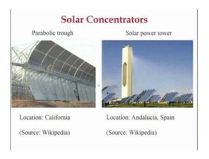
And solar energy can also be used in the form of solar concentrators. So, in the previous case, the energy of the area of the collector is equal to area of the receiver, because it is a flat panel. What happens in concentrator is we use a curved surface which is a reflecting surface. So, area of receiver is far higher as compared area of he reflecting surface, but area of the surface which receives the sunlight is the curved surface is very large.
