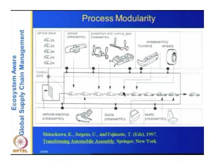
Now what about process modularity? The assembly process modules are shown here. These two diagrams illustrate the product and process modularity for automobile manufacture
