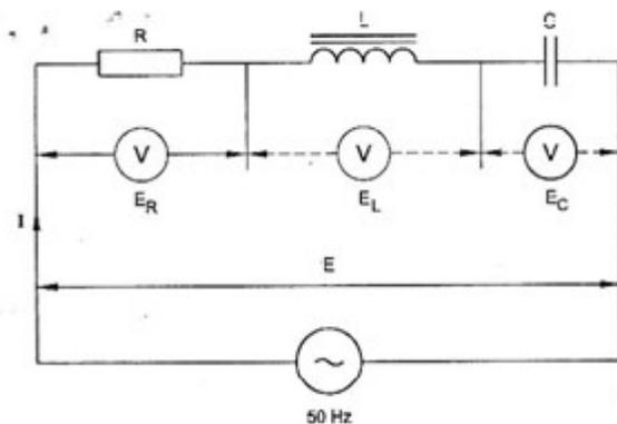
**Current**  $I = \text{Voltage} / \text{Impedance} = E / Z$
