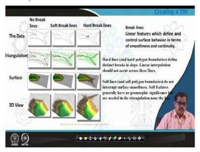
So I have just given you a representation of this, this was actually adapted from young core wherein this entire description of this particular image gives you exact way of how a 3D view is developed. First, the triangulation is developed, then how the surface is developed and finally the 3 D view is developed. The first thing that we have to understand as brake lines.
