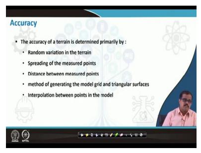
So, coming to accuracy, accuracy of the terrain is determined primarily by various issues. One is random variation in the terrain, how random is the variation in that particular terrain, then the spreading of the measure points. So, have you collect, how was the points been mentioned in the entire model, is it mentioned as a group in certain corner or is it has a random measurement all throughout the place or it you have points all throughout your place.
