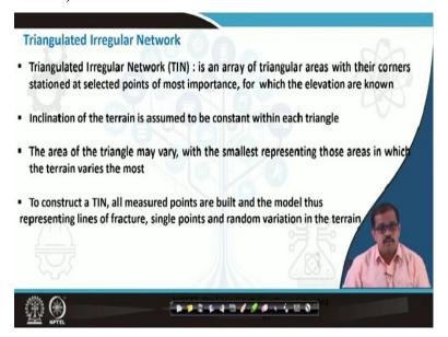
Triangular irregular network it is actually an array of triangular areas. So, when I say triangular areas it is an enclosed polygon okay with their corners station at select selected points of most importance for which elevations are known. Please be careful of this, when I say most important it does not mean that it is an important place on the surface, it means to say that where we know the values that point on the earth's surface is selected as a nodal point.
