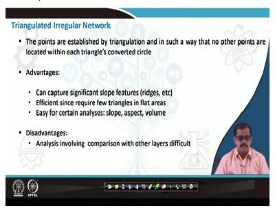
So the points are established by if I have to define TIN in a very simpler way. The points are established by triangulation and in such a way that no other points are located with each triangles that is converted to circle, that is what I mean by the previous one. So I have already said what are the different advantages and what the only disadvantage that we find delaunay triangulation is analysis involving the comparison with other layers is extremely difficult.
