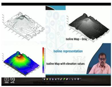
Now, so these are some of the isoline representation, so can see this is the elevation values have been added here, you can see these are the elevation we have generated a thematic map so that you understand this and this is a normal isoline representation and this is in the great value shades. So you can see the lighter shades actually representing and elevation that this at a very high elevation and the ground at a lower evaluation is represented in grey complete grey or closer to black.
