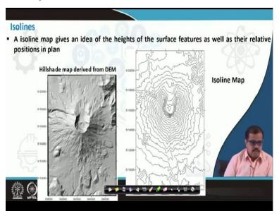
So and it also gives an idea of height that is why we use of isoline in wherever you need the idea of height you can use an isoline a surface features as well as relative position in the plan is shown. For example here this is an hill shade map that has been developed from the DEM, will also develop the hillshade map in our practical classes, when we look at this hill shade map or you can see various features on the ground that has been denoted.
