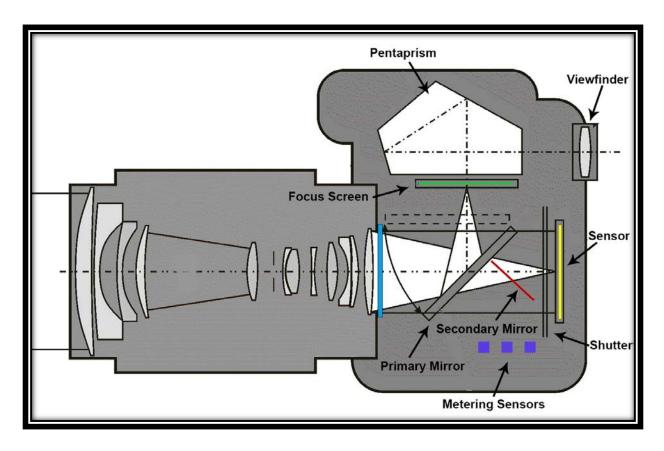
The mirror in front of the sensor needs to move up and out of the way to expose the sensor. There is also a secondary mirror behind the primary mirror.
