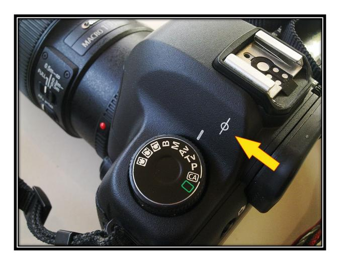
There is a special icon on SLR cameras (film and digital) which is a circle with a line through it which indicates the location of film plane, or the sensor of the body. This is useful if you are making a pinhole camera or modifying the length of the lens of the camera body itself.
