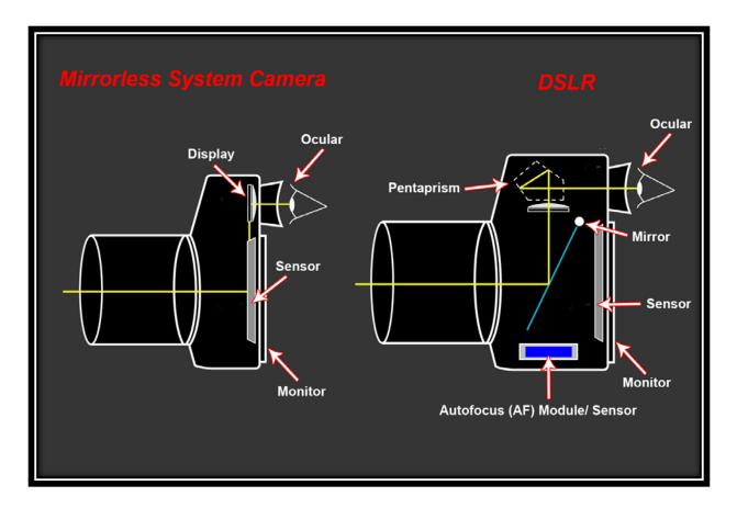
Mirrorless and Bridge cameras do not have mirrors inside them. Instead, they have an Electronic Viewfinder (EVF). When light passes through the lens of these cameras, it goes straight to the imaging sensor. The sensor sends a signal to the viewfinder and we can see the image through this.
