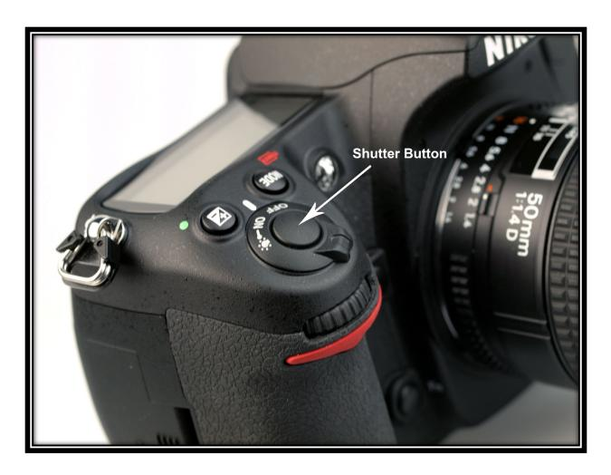
They will also have a Shutter Button which is used to take the photograph. This is also called the Exposure Button.
