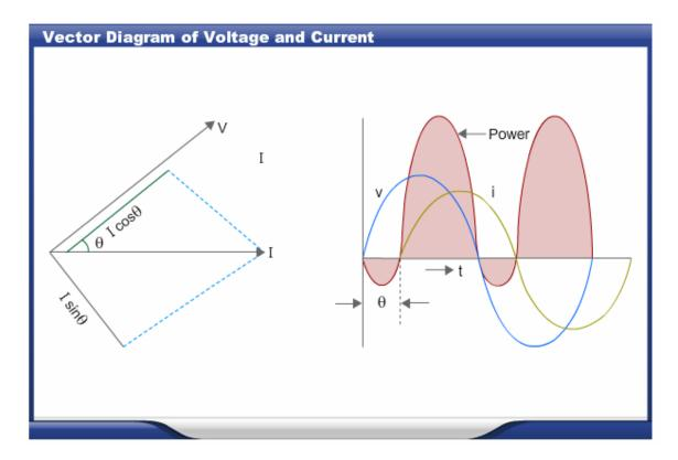
The power consumed is given by the product of V and I cos $\theta$  component of the current I, which is in parallel or in phase with the voltage V.
