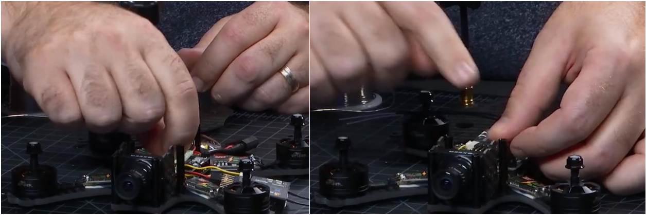
Use double sided tape to stick down the transmitters receiver.
