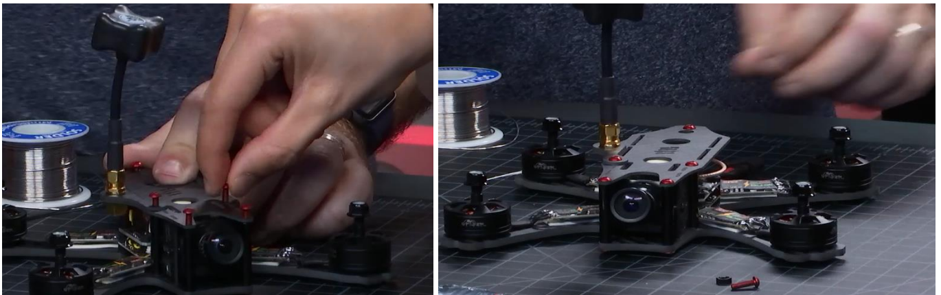
Screw in the top plate. You have finished putting together the main parts of the drone.
