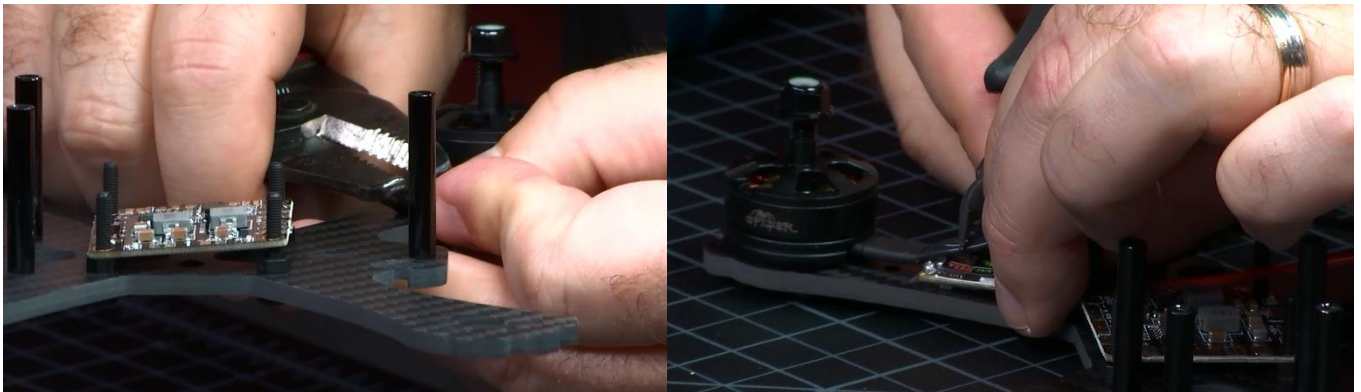
Trim motor wires for attaching to the electronic speed controller.
