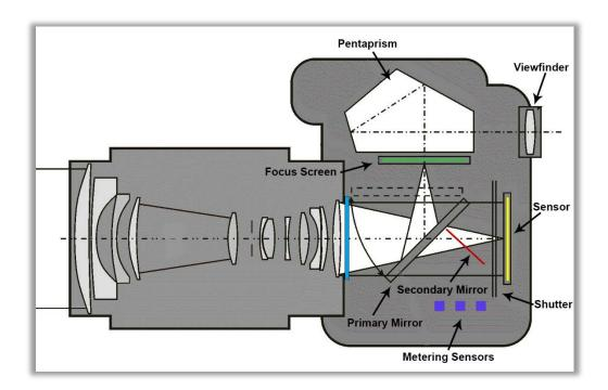
When you're adjusting your settings in shutter priority mode, what you're really adjusting is the duration that the curtain is open, exposing the sensor to light. The shutter settings control the exact duration for how long this shutter curtain is open.
