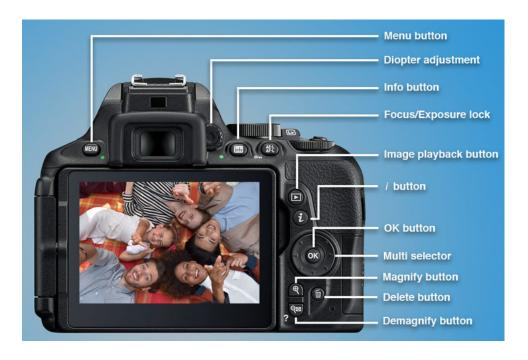
Commonly-used controls on the back of the camera include:
