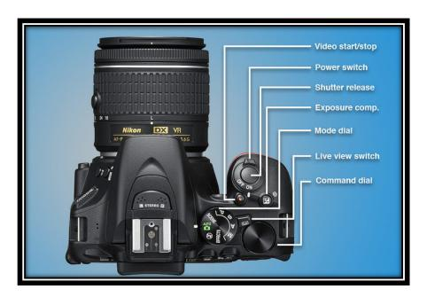
Commonly-used controls on the top of the camera include:
