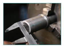
The boring tool bar should be clamped as close to the holder and tool post as possible considering the depth of boring to be done. The bar will have a tendency to spring away from the work piece if the bars over hangs the tools post too far. If deep boring is to be performed, it will be necessary that the bar is as thick as possible to counteract this springing tendency.
