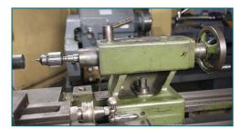
1. Mount the center on the tailstock.
