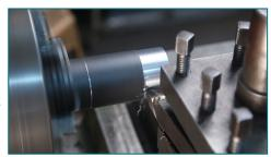
The tool cutting edge should be sharp and ground to the recommended rake and clearance angles. Depending upon the material to be turned and the tool material, the recommended cutting speed is to be chosen from the chart available, to determine the spindle speed for plain turning. The selection of the recommended feed rate is also important which greatly depends upon the depth of cut and the cutting speed chosen.
