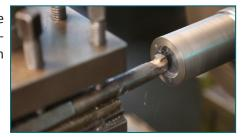
**Mohan**: Boring is used to achieve greater accuracy of the diameter of a hole, and can be used to cut a tapered hole. Boring can be viewed as the internal-diameter counterpart to turning, which cuts external diameters.
