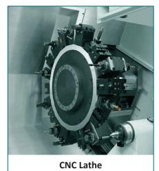
The setting has to be done in such a way that irrespective of the tool being on turret it comes to the point of operation. The setting must be done specifically for this operation and this tool.
