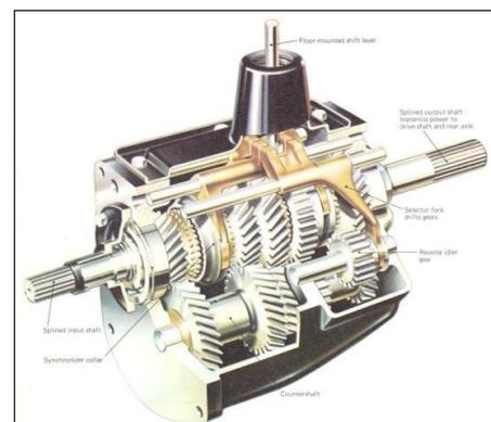
◆ Synchronmesh type transmission.
