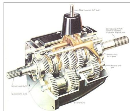
◆ Synchronmesh type transmission.
