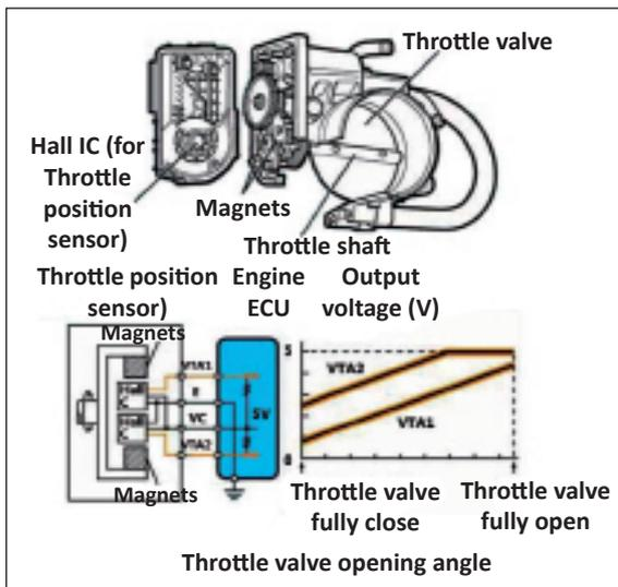
This sensor not only accurately detects the throttle valve opening, but it also uses a non-contact method and has a simple construction, so it does not break down easily. In addition, to maintain the reliability of this sensor, it outputs signals from two systems with different output characteristics.
