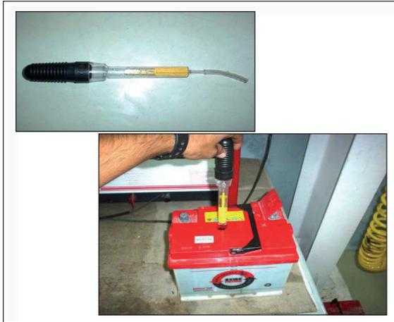
Hydrometer is used to check the specific gravity of electrolyte solution of battery.
