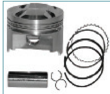
Usually three in numbers and the top two are compression rings and the bottom helical one are oil rings. The piston pin is made up of steel and has two locks to keep the piston in place and connected to the connecting rod.
