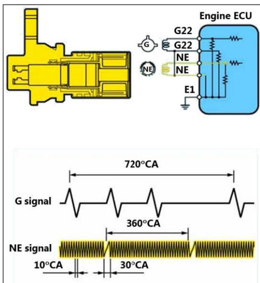
The engine ECU uses the NE signal and G signal to calculate the basic injection duration and basic ignition advance angle. As with the G signal, the NE signal is generated by the air gap between the crankshaft position sensor and the protrusions on the NE timing rotor periphery installed on the crankshaft. The illustration shows a type of signal generator with 34 protrusions on the NE timing rotor periphery and an area with two teeth missing.
