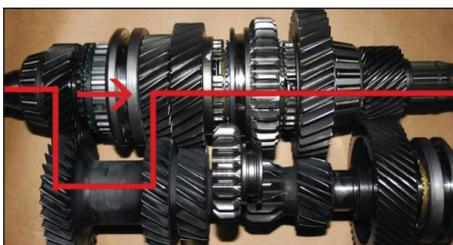
When the shift from second to third gear is made, the shift fork returns the first/second synchronizer to its neutral position.
