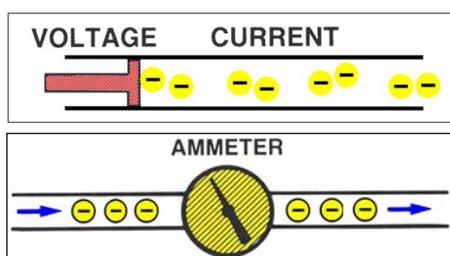
Current can be described as the rate of electron flow. It is measured in amperes. The current increases as pressure or voltage is increased – provided that circuit resistance remains constant. Another term for amperes is 'intensity of current'. The symbol for current intensity is  $I$ . The symbol for amperes is  $A$ .
