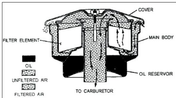
Figure 4-15,–Wet-type air filter
