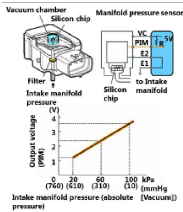
The manifold pressure sensor is used with D-type EFI for sensing the intake manifold pressure. This is one of the most important sensors in D-type EFI. By means of an IC built into this sensor, the manifold pressure sensor senses the intake manifold pressure as a PIM signal. The engine ECU then determines the basic injection duration and basic ignition advance angle on the basis of this PIM signal.
