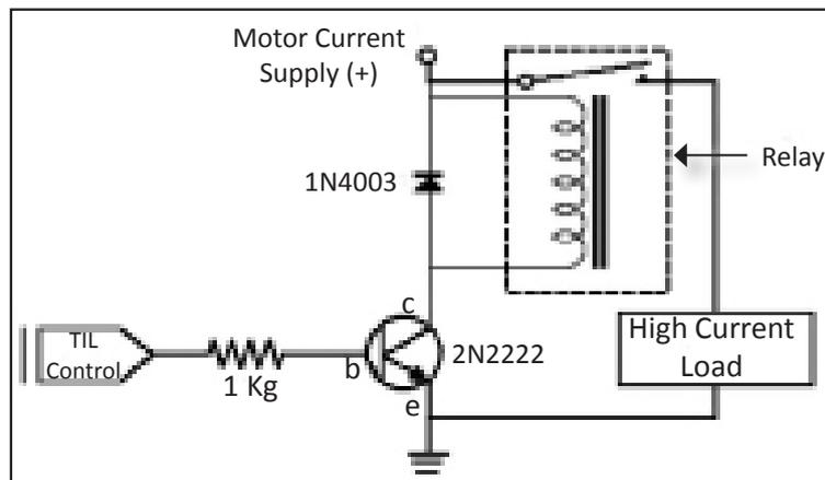
A transistor performs the same function as a relay. It does not wear out and is therefore non-wearing. In addition to that a considerably higher switching frequency is possible, for example for fuel injection valves.
