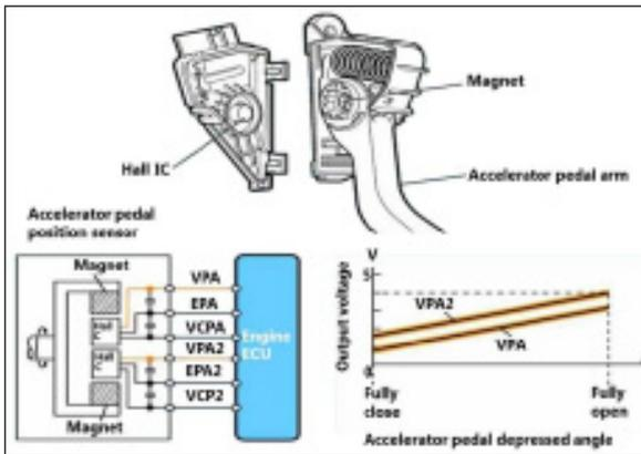
**Accelerator Pedal Position Sensor:**
