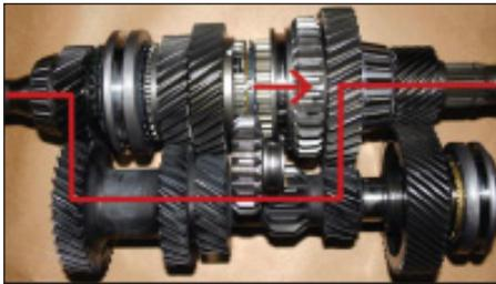
In first gear position, the power enters the transmission through the main shaft and is transmitted to the lay shaft since the main shaft gears are in constant mesh with the gears on the lay shaft.
