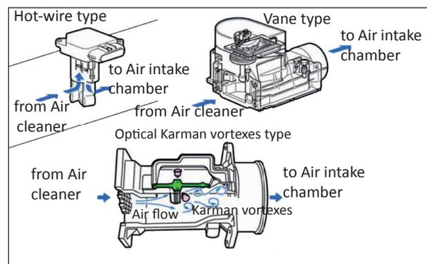
Currently, most models use the hot-wire type of air flow meter because it has superior measurement accuracy, lighter weight, and better durability.
