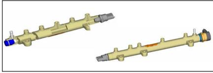
Common rail or high pressure accumulator receives fuel at high pressure from the high pressure pump. The rail stores and distributes the fuel at individual injectors. It also helps in dampening the pressure vibrations caused by the high pressure pump and the injection process. The fuel rail pressure during engine idling and running temperature condition ranges approximately from 300-400 Bar and ranges to a maximum value of 1600-2000 Bar.
