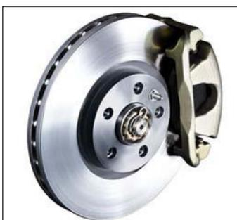
Brakes are vital components in an automobile. The primary function is to reduce the speed of the vehicle in order to prevent accidents. Automobiles are generally equipped with disc brakes in the front and drum brakes at the rear. However, some automobiles are also available with all four disc brakes too.
