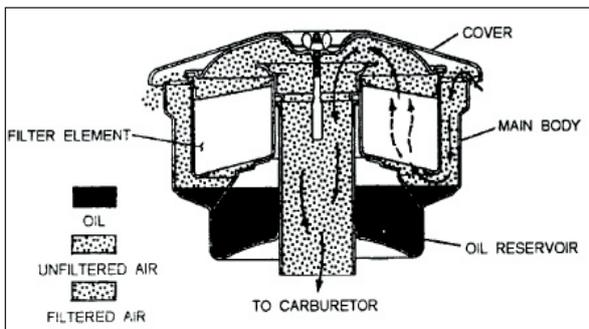
Figure 4-15,–Wet-type air filter
