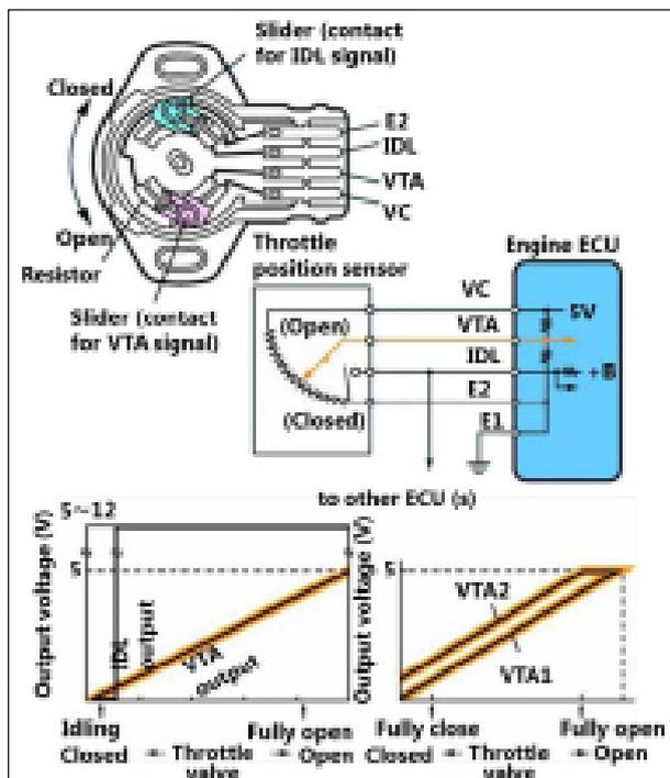
**Throttle Position Sensor: Linear type**
