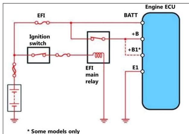
Battery voltage is supplied at all times to the BATT terminal of the engine ECU to prevent the diagnostic codes and other data in its memory from being erased when the ignition switch is turned off.
