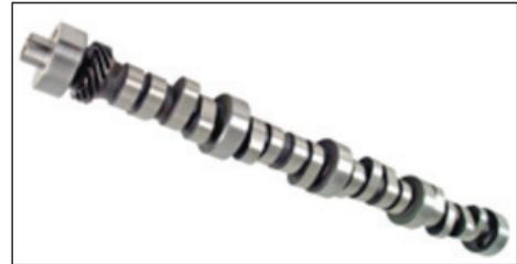
Engines can be equipped with single overhead cam shaft (SOHC) or double overhead camshaft (DOHC)
