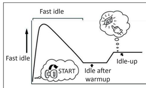
The ISC system controls the idle speed so that it is always appropriate under varying conditions (warm-up, electrical load, etc.).
