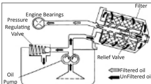
In a full flow system the oil passing through the engine bearings and galleries passes through the oil filter first. In the case of blocking of the oil filter occurs, the engine bearing will be starved from lubrication which could lead to seizing of engine.
