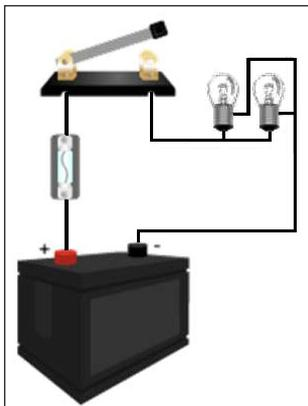
The parallel circuit has two or more paths for electrons to flow. Current in this circuit is shared between the branches.
