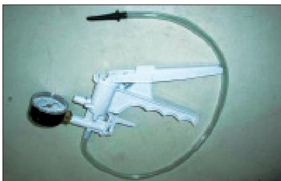
Vacuum pump is used to create vacuum pressure at any component, which works on vacuum and measure the voltage output or functional operation. For inspection of MAP sensor [as shown in the picture] the gauge needs to be connected to with sensor and by creating a vacuum pressure. The output voltage of the sensor is notified on the multimeter.
