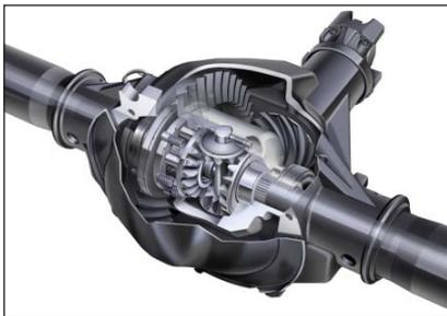
A differential is a gear mechanism that is housed in the transaxle in the case of front wheel drive vehicle or in the rear axle in the case of a rear wheel drive vehicle. The main function of a differential is to differentiate the speed of the inner and outer wheels while on a turn to prevent skidding.
