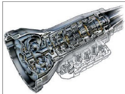
Transmission is a solid robust device that is made up of gears of different sizes mounted on parallel shafts. It is situated between the clutch and the driveshaft in the case of a front wheel drive vehicle and clutch and the propeller shaft in a rear wheel drive setup. It works on the principle of gearing, in which a set of gears mesh together to provide the desired output speed. The output speed also depends on the gear ratio of the meshing gears.
