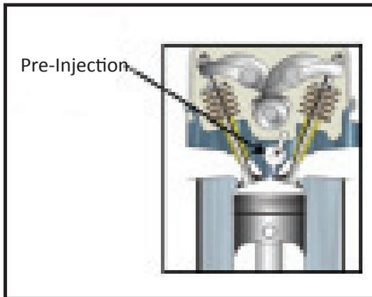
Here fuel is injected into a small pre-injection chamber which is connected to the cylinder by a narrow opening. The initial combustion takes place in this pre-chamber slowing the rate of combustion
