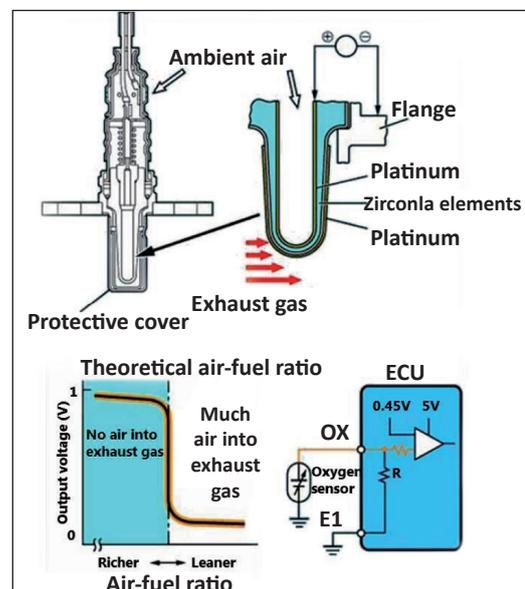
At high temperatures ( $400^{\circ}C$  [ $752^{\circ}F$ ] and higher), the zirconium element generates a voltage as a result of the large difference between the oxygen concentrations on the inside and outside of the zirconium element.
