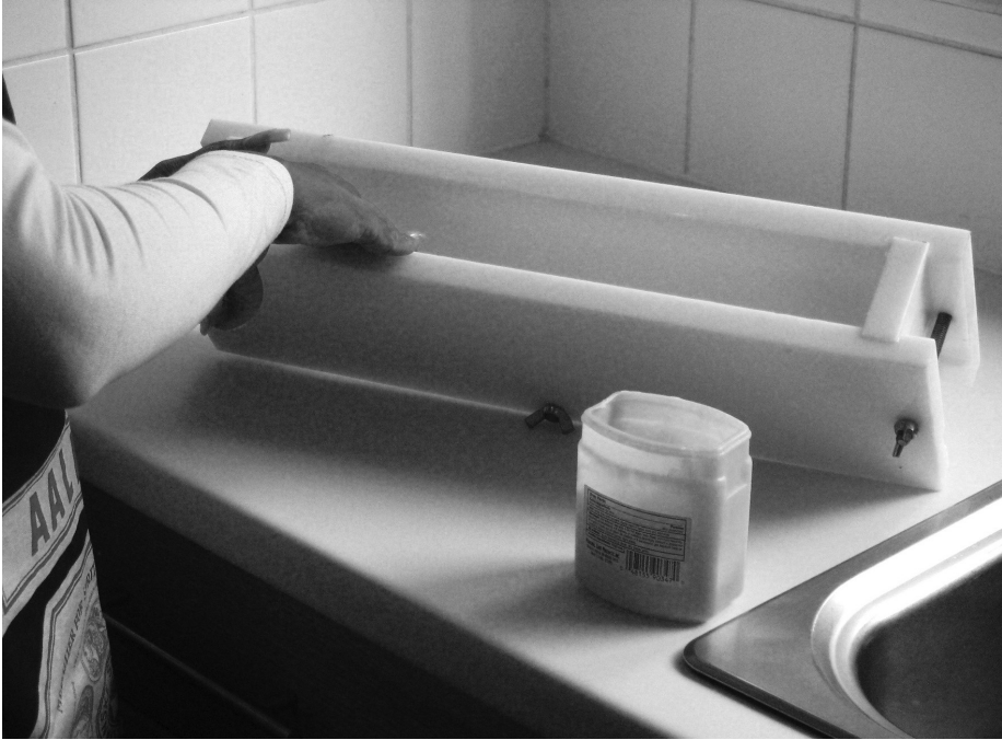
fig 28: grease all sides of the mould
