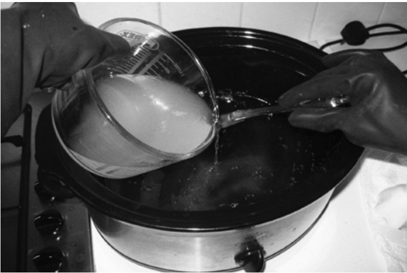
fig 32: add the caustic solution to the heated fats and oils
