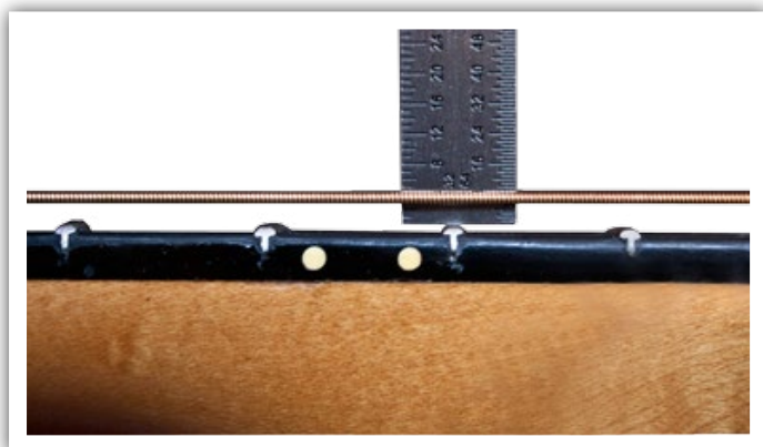
"Guitar action" is the distance between the fretboard and the strings.
