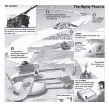
The dismal failure of a British built drone during the war in Iraq has led the Ministry of Defence to reconsider its plans for a futuristic fleet of unmanned aircraft. Britain lost 23 of its Phoenix surveillance planes, which each cost about £1.5m.
