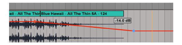
This will reduce the volume of the track so it fades out. You can repeat the process with the second track so that it fades in.
