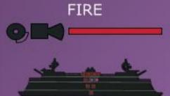
The general alarm bell rings continuously for more than 10 secs followed by 1 to 4 short rings indicating the fire location by deck level, supplemented by the same signal on the ship's whistle
