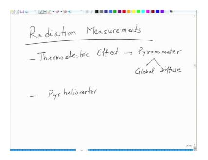
So, how you do the radiation measurement? Radiation measurement is done by basically based on thermoelectric effect. And for this we use equipment called as Pyranometer. And this can measure both global and diffused radiation. And the second one is called as Pyrheliometer. These are the two equipments which are used for measurement of radiation.
